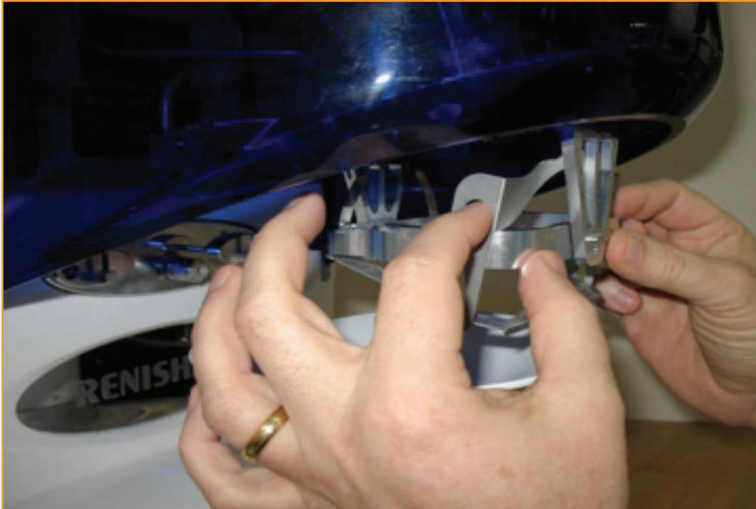
3. Load the billet with the chamfered corner to the left and the flat edge towards the front of the machine.
