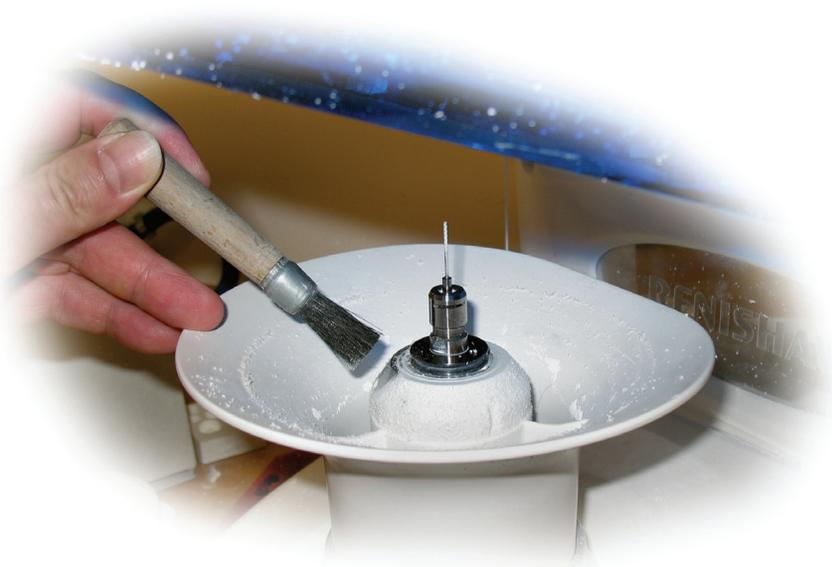
2. Remove the collet and tool holder. Clean the dust out of the collet and the spindle.
