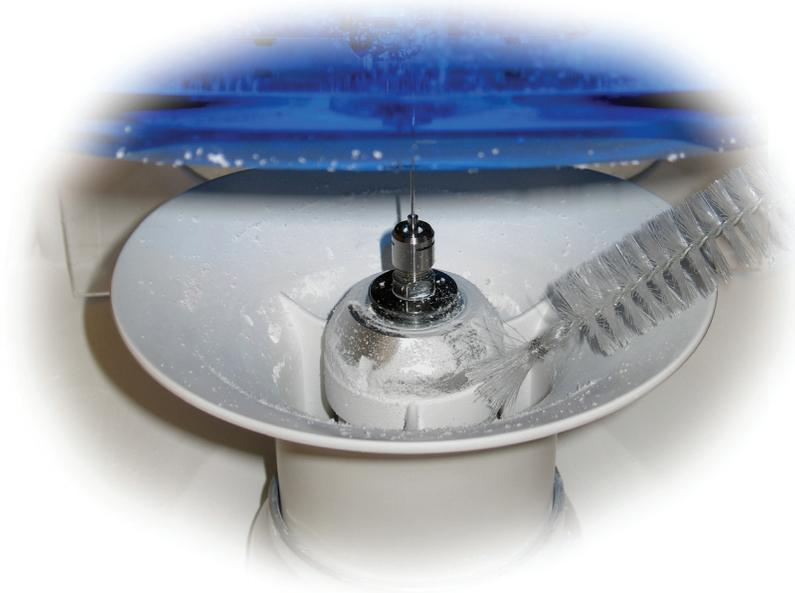
2. Clean inside the shroud until you reach the bottom of the tube which will be approximately the full length of the brush. This process is required to ensure that the build up of zirconia dust does not become excessive and prevent effective dust extraction.
