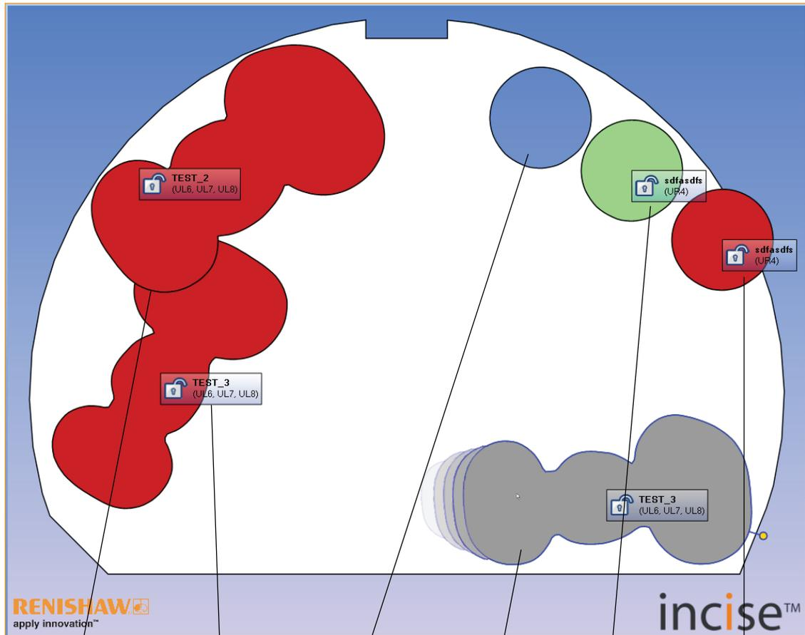
Frameworks overlapping - position not OK      Framework identifier and status      Framework that has been marked as cut out      Framework grey when being moved      Framework positioned correctly      Frameworks overlapping billet edge - position not OK
