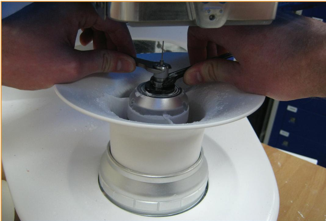
2. Hold the spindle with the bottom spanner and slacken the collet with the top spanner until the tool is free to be removed.
