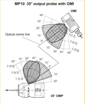
Switch-on/off range The OMP must be within 3 m (9.8 ft) of the OMM. Operating range The OMP must be within 6 m (19.6 ft) of the OMM. Range metres (feet)
