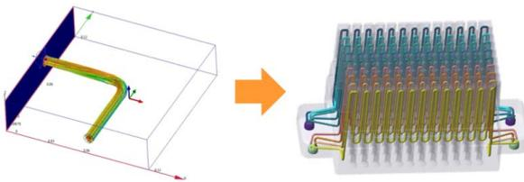
An irregularly shaped mould tool can also be cooled using multiple channels of equal diameter and length. In this instance, eight cooling channels, each 3 mm in diameter and of equal length, have been built into the mould tool. All eight channels are connected to 10 mm diameter inlet and outlet ports to guarantee equalised flow.
