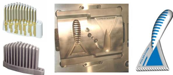
It should be noted that an AM process will not produce surfaces of sufficient quality for many moulding applications. Most AM moulds are finish machined and polished to produce the desired surface precision.
