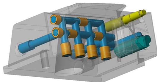
Additive manufacturing (AM) frees us from the constraints of cross drilling. Now we can design internal channels that follow the surface of the tool, and which have smooth corners for faster flow, increasing the heat transfer into the coolant. In the example below, we have separate cooling circuits for different areas of the slider, designed to carry the heat away at a consistent rate to promote even cooling.
