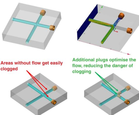
This approach has its limitations when we are designing a conformal-cooled slider, as shown below. The channel network is limited in its shape so that it sits deeper below the surface of the tool, making cooling less efficient. Not only that, but we also have to deal with additional machining and
