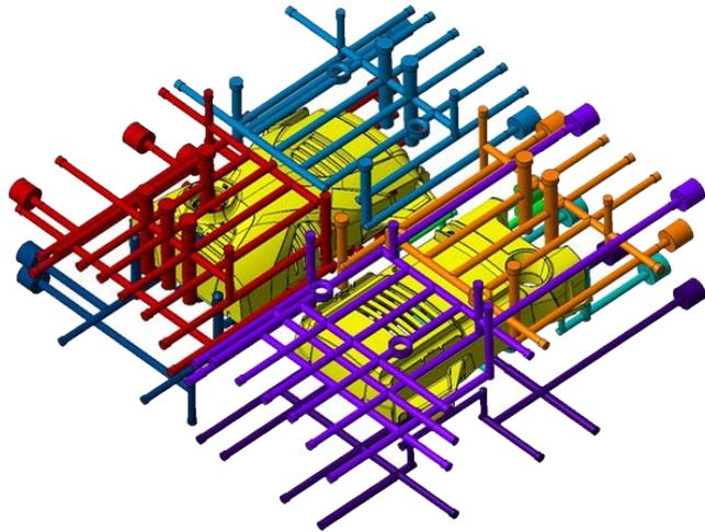
assembly time, as well as dead-spots in the channel network that may clog up over time. In complex cases, conformal cooling channels can only be inserted by producing the tool in sections, resulting in extra joints that can shorten the life of the tool.
