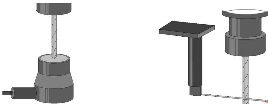
Conventional non-contact tool setting systems use a beam of laser light passing between a transmitter and a receiver, located either on the table of the machine, or on each side of it so that the beam passes through the working volume.
